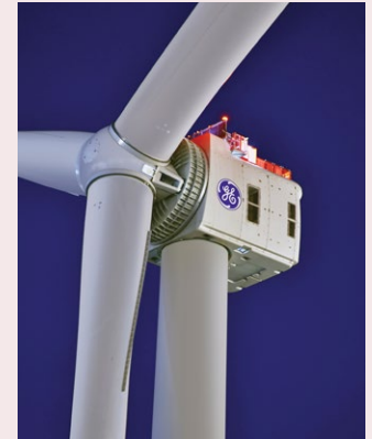
Prototipul Haliade-X 12 MW Photo: General Electric
